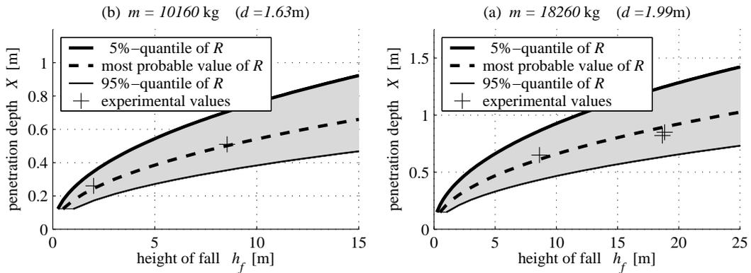
Figure 1: Comparison of model results (eqns (1)–(3) with  $R = R_{5\%}$ ,  $R = R_{50\%}$ ,  $R = R_{95\%}$ ) and experimental results for (a) the  $18260\text{ kg}$  rock boulder and (b) the  $10160\text{ kg}$  rock boulder
