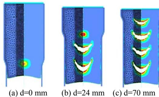
Figure 2. Numerical prediction of the discontinuous chevron cracks in forward cold extrusion of a cylindrical bar without adaptive remeshing but with kill element procedure.
