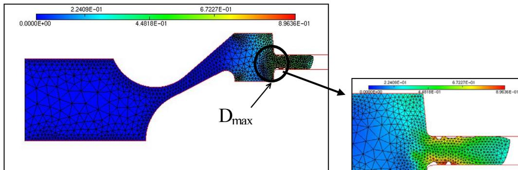
Figure 2 : Damage distribution at the end of the operation for  $u=14.75$  mm
