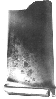
Figure 1: Bottom part of the fractured blade.
