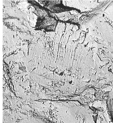
Figure 3: Fatigue striations in the biode-carbon replica of the fracture surface ( $a = 10$  mm, 10000x)
