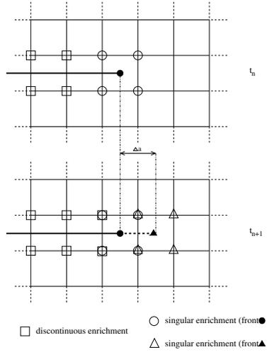
Figure 1. Strategy for enrichment when the crack propagates
