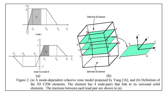
During a deformation process, displacement increments will be passed on to the cohesive element, within which the separations and tractions are updated according to the cohesive laws. The updated nodal force vectors and stiffness matrix are then added to the global stiffness matrix to check the total force balance. Iteration continues until an equilibrium condition is satisfied for each displacement increment.
