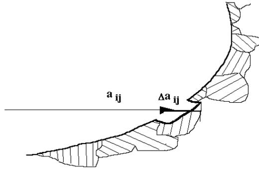
Figure 1: Microstructural configuration at the crack front: The crack front cuts many grains with different orientations and grain length; the crack is moving in one crack front segment  $a_{ij}$  by  $\Delta a_{ij}$ .
