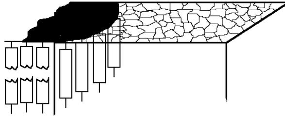
Figure 2: Micromechanical configuration at the crack front and the modeling with single elements
