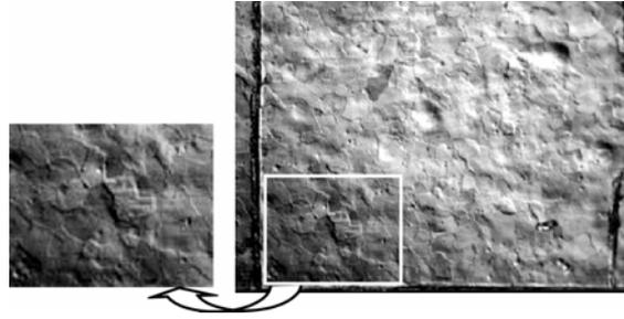
Figure 3: The surface structure of the recrystallized VT1-0 titanium specimen,  $N = 20 \times 10^6$  cycles;  $\times 500$
