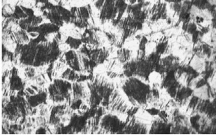
Figure 2: The mesostructure-II in the aluminum specimen surface.  $N = 5 \times 10^6$  cycles. Designated by numbers are the self-consistently deforming grains within the conglomerates;  $\times 100$
