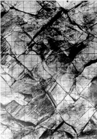
Figure 1: The large-scale rectangular mesostructure-II in the lead specimen surface layer,  $N = 5 \times 10^3$  cycles;  $\times$
