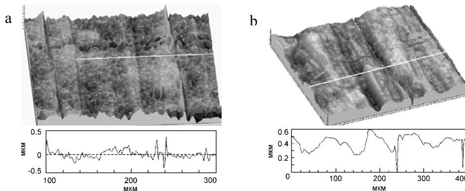
Figure 4: The surface roughness and the corresponding cross profile of the recrystallized titanium specimen tested in alternating bending: coarse-grained surface,  $N = 20 \times 10^6$  cycles (a); nanostructured surface layer,  $N = 14.5 \times 10^6$  cycles (b);  $\times 500$
