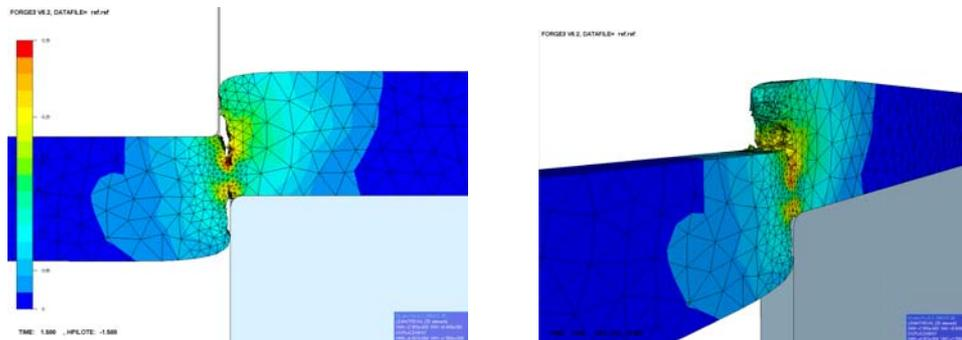
Figure 1. Blanking simulation: isovalues of damage during fracture
