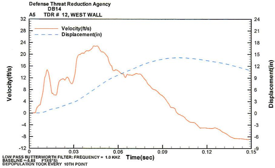
Figure 4. Actual velocity and displacement vs. time during blast
