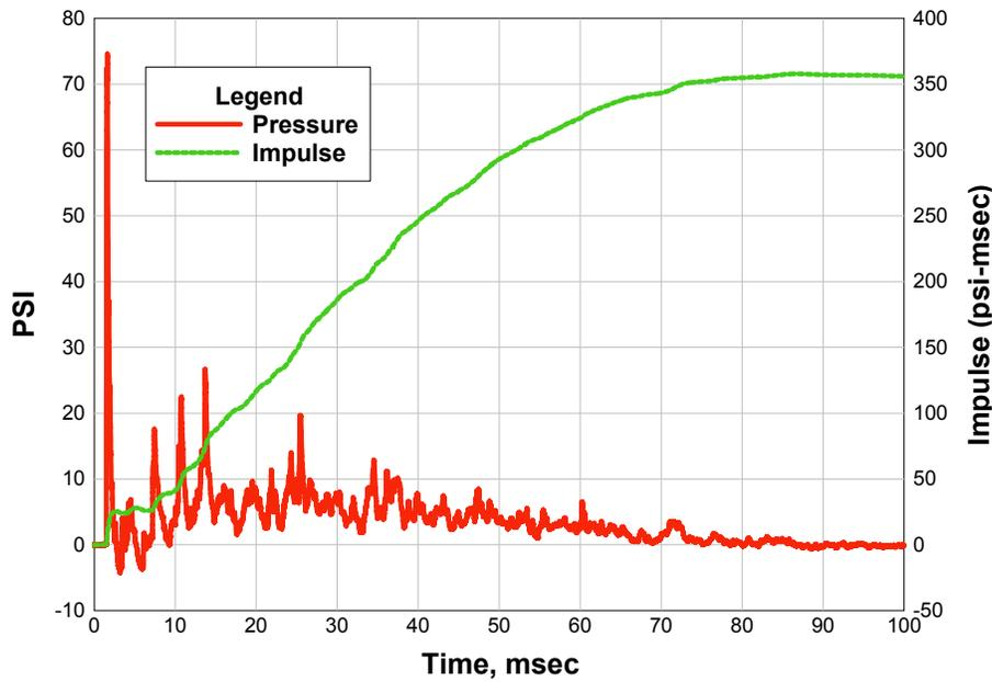
Figure 3. Measured blast pressure vs. time
