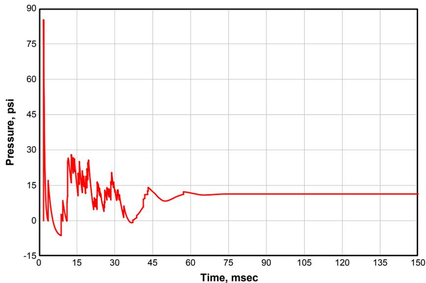
Figure 1. Predicted Pressure-time by BLASTX
