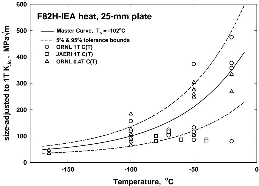
Figure 1: Size-adjusted to 1T fracture toughness data of F82H plate relative to its master curve and 5% and 95% tolerance bounds.
