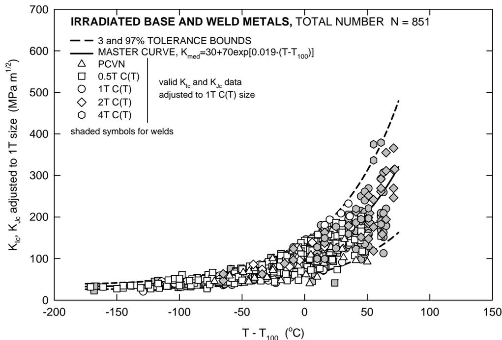
Figure 2: Fracture toughness of large number of RPV steels plotted against reference temperature,  $T - T_0$ , relative to the master curve from Ref. [2].
