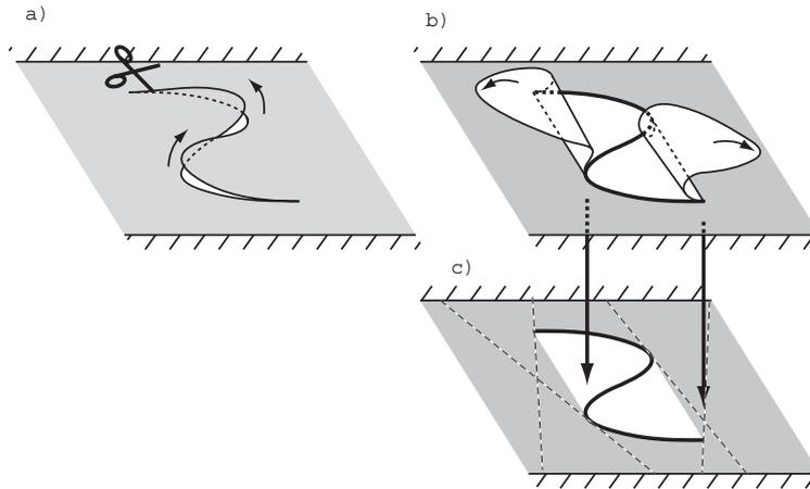
Figure 2: For a given fracture path, (a), in a thin sheet clamped along its lateral edges, the “soft zone” is defined as the area that can be deformed by pure bending, (b), that is with a negligible elastic energy. This soft zone, shown in white is the convex hull of the crack path. (c) The model operates on the two dimensional projection of the strip rather than on the full three dimensional configuration.
