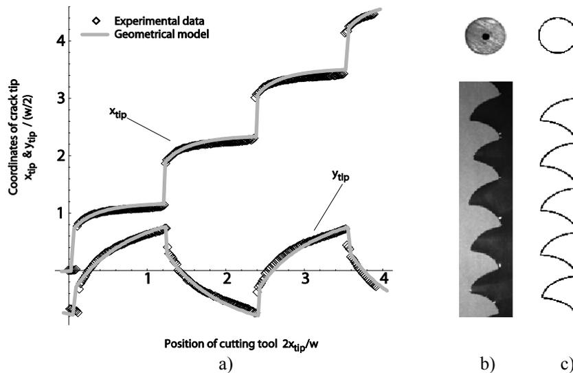
Figure 4: (a) Time-series for the coordinates of crack tip (i.e. as a function of tool position since cutting speed is constant.  $x_{tip}/y_{tip}$  along/perpendicular to the direction of cutting. Experimental (black symbols) and model prediction (solid grey lines). (b) : Experimental (b) and numerical (c) crack morphologies, for the same cylindrical cutting tool (circles with 31mm diameter, on top).
