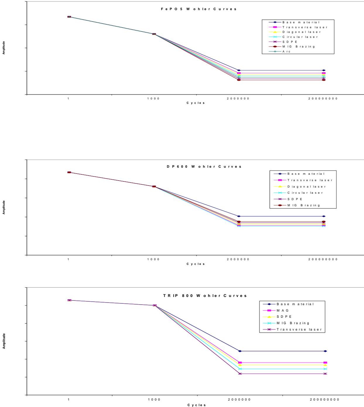
Figs. 7 Wohler curves of FePO5, DP600 and TRIP 800 steels after different welding conditions
