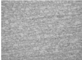
Microstructure composed of ductile ferrite matrix containing small islands of hard bainite and retained austenite, fig.3. Transformation of retained austenite to martensite during deformation causes significant strain hardening and retards the onset of necking. Efficient strain redistribution during forming (hence good drawability) combined with high yield strength and energy absorption in the finished component, make these steels suitable for structural and reinforcement parts.
