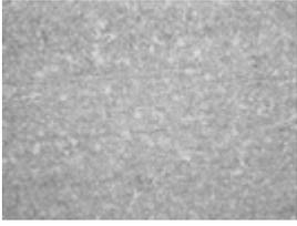
Microstructure consisting of a fine dispersion of hard martensite particles in a pure ferrite matrix, fig.2.
