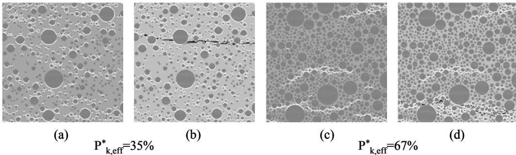
Figure 2: Crack patterns at peak, (a) and (c), and 25  $\mu\text{m}$  displacement, (b) and (d)
