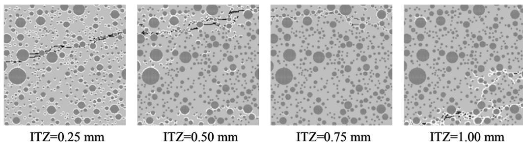
Figure 4: Crack patterns at 25 μm displacement
