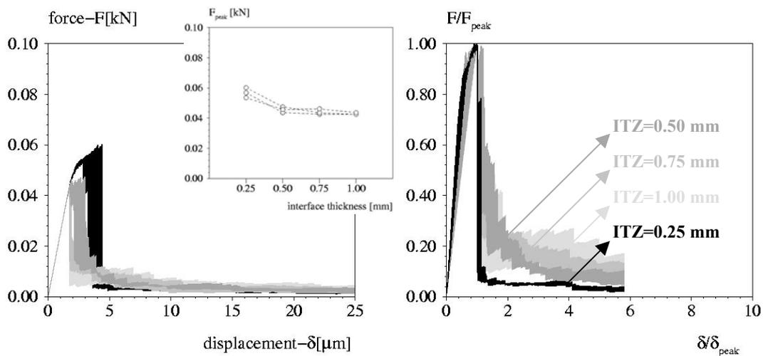
Figure 3: Results for different interface thicknesses
