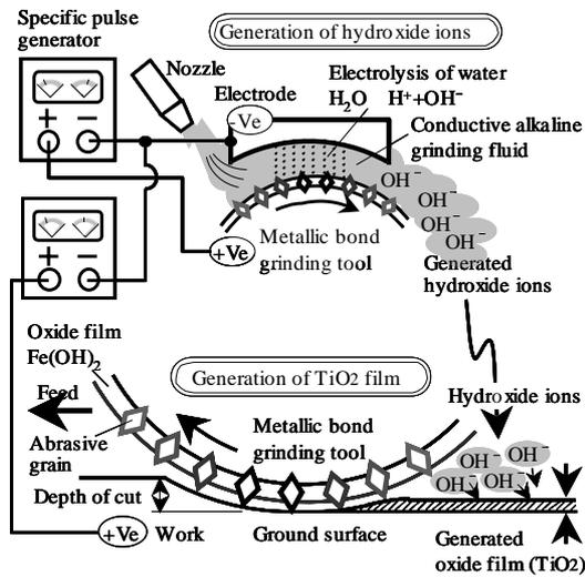
Fig. 1 Schematic illustration of a new ELID grinding system
