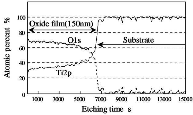
Fig. 3 Titanium and oxygen profile in the depth direction of the Ap-ELID series
