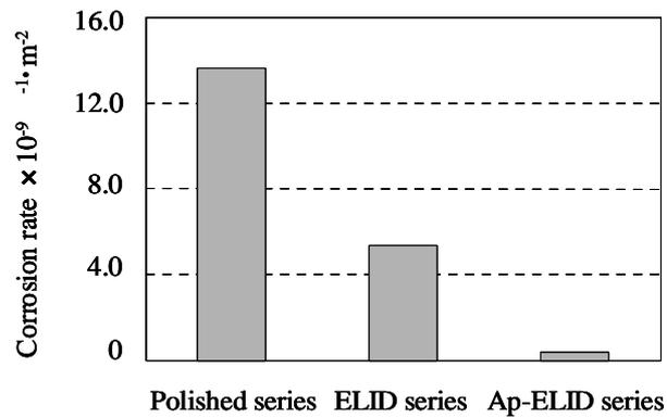
Fig. 4 Comparison of the corrosion rate
