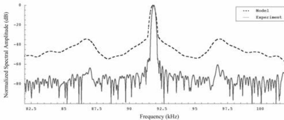
Figure 3: Comparison of the frequency spectrum of a bi-tonal signal generated by the discussed model and by AMA testing
