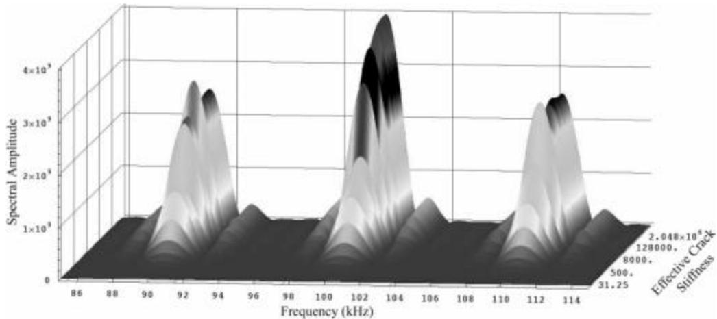
Figure 2: Frequency spectrums of model generated bi-tonal signal with increasing effective crack opening stiffness and no external closing pressure
