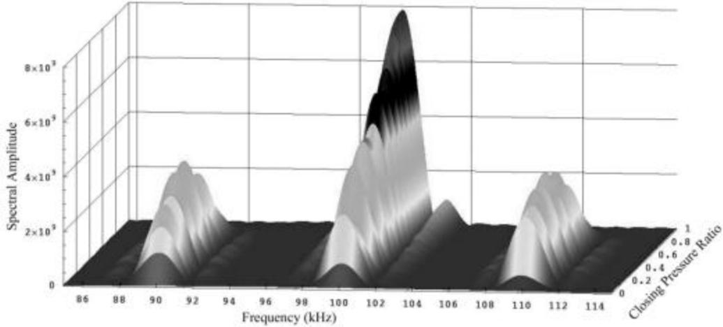
Figure 1: Frequency spectrums of model generated bi-tonal signal with increasing external pressure and no crack separation dependency
