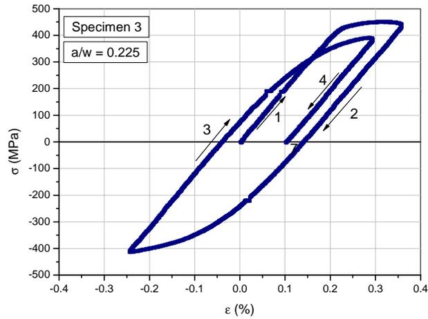
Figure 2: Stress vs. Strain diagram for SENT specimen. Short Crack.
