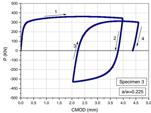
Figure 3: Load vs. Displacement diagram for SENT specimen. Short Crack.
