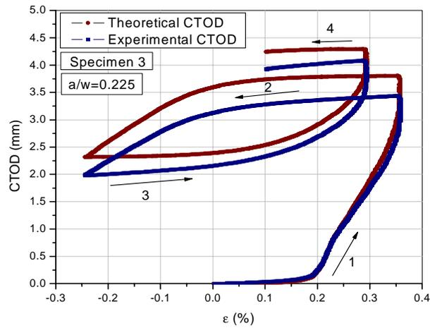
Figure 4: Comparison Experimental / Theoretical CTOD vs. Strain diagram. Short Crack.
