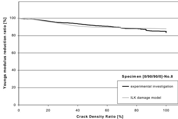
Fig. 4: Crack density studies: experimental and theoretical elastic moduli reduction
