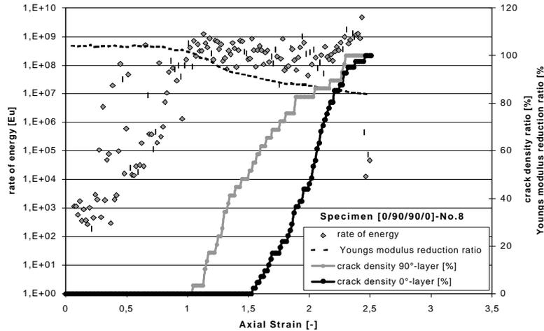
Fig. 3: Experimental data: Youngs modulus reduction, crack densities and acoustic emission data as a function of axial strain
