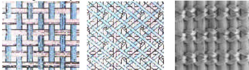
Fig. 1: braided/woven fabric; warp knitted fabric; weft knitted fabric
