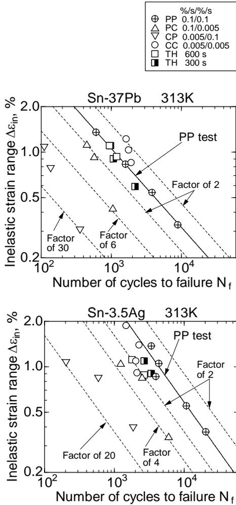
Fig. 6 Correlation of creep-fatigue lives in the five strain waves with inelastic strain range.
