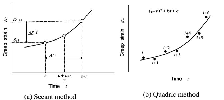
Fig.2 Method for calculating creep strain rate.
