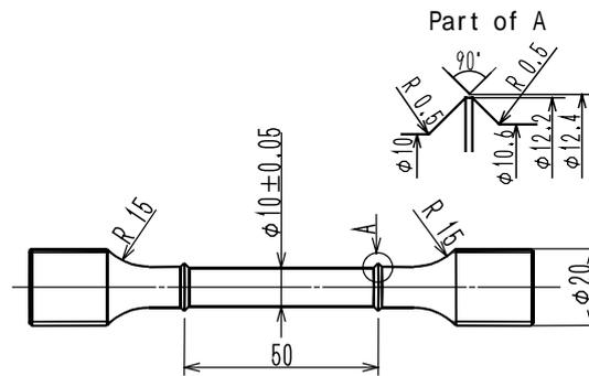
Fig.1 Shape and dimensions of creep specimen.
