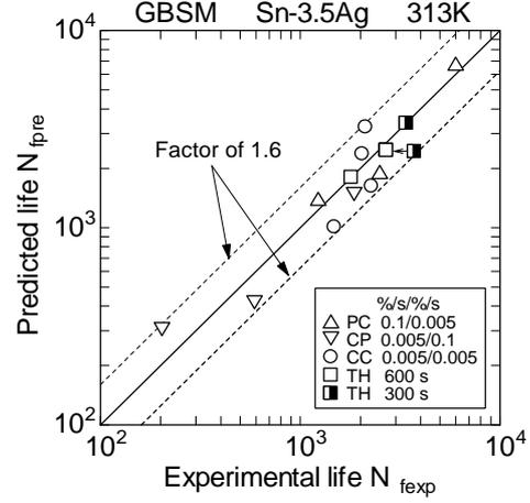
Fig. 8 Correlation of creep-fatigue lives with the grain boundary sliding model.
