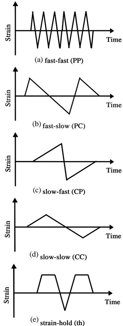
Fig. 5 Five strain waves for creep -fatigue tests.
