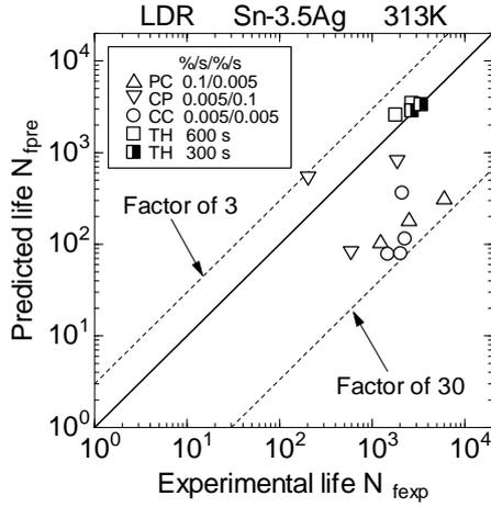
Fig. 7 Correlation of creep-fatigue lives with the linear damage rule.
