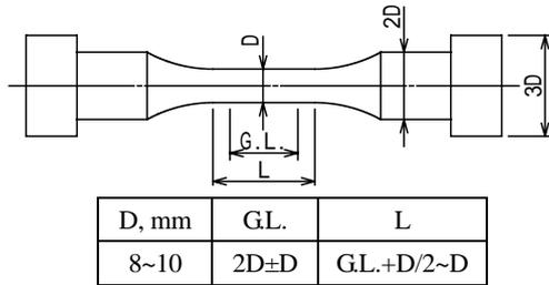
Fig.4 Shape of creep-fatigue specimen
