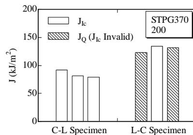
Fig. 2  $J$ -integral values for specimens subjected to fracture surface analysis[8].
