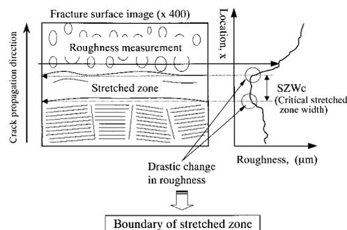
Fig. 1 Outline of  $SZW_C$  measurement by proposed method
