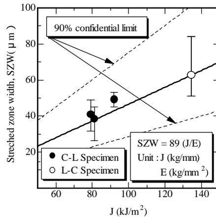
Fig. 4 Relationship between  $J$ -integral and stretched zone width evaluated by proposed method.
