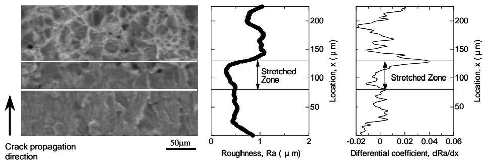
Fig. 3 Quantitative evaluation result of  $SZW_c$  by proposed method (C-L specimen,  $J_{Ic} = 79.1 \text{ kJ/m}^2$ ).
