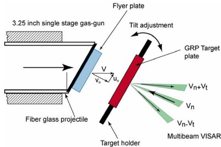
Figure 2: Schematic of the Gas Gun pressure-shear plate impact experiments.
