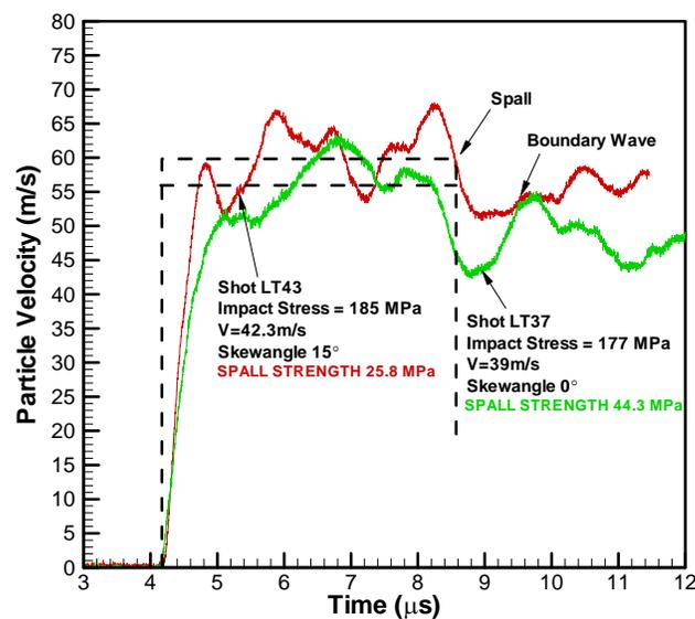
Figure 4: Spall Experiments for GRP composites under Normal Compression and 15 degree Pressure-Shear Shock Loading.
