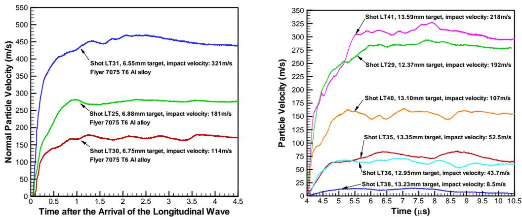
Figure 3: Structure of shock wave at three different impact speeds -- 114 m/s, 181 m/s and 321 m/s. The thicknesses of the GRP target plate for the three cases are 6.75 mm, 6.88 mm, and 6.55 mm, respectively.
