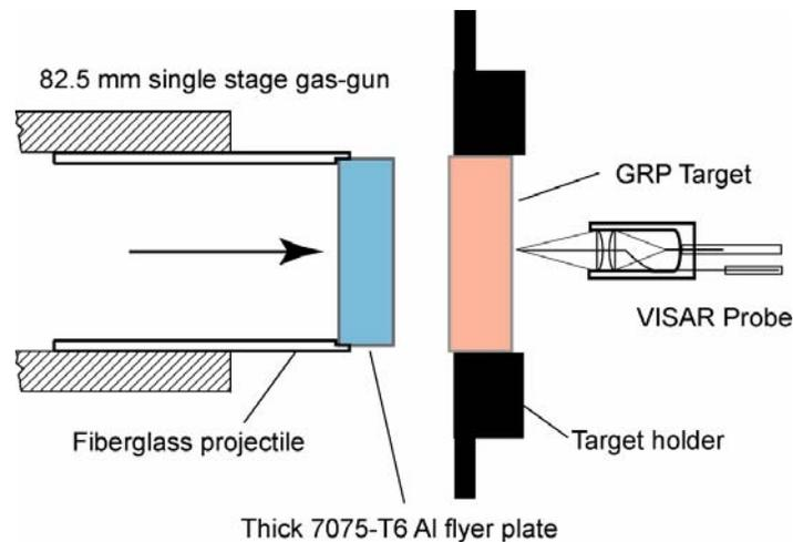
Figure 1: Schematic of plate impact experiment used to study structure of shock waves during shock compression.
