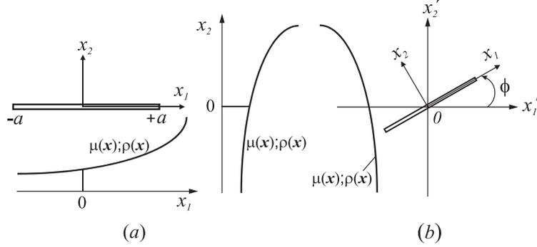
Fig. 1: An infinite FGM containing a finite crack
