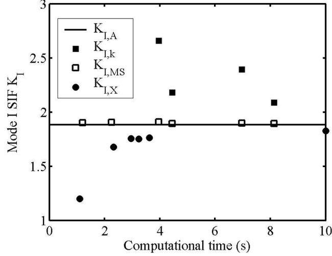
Figure 4: Comparison of the values of the stress intensity factor  $K_I$  calculated using various methods as a function of the computational time.
