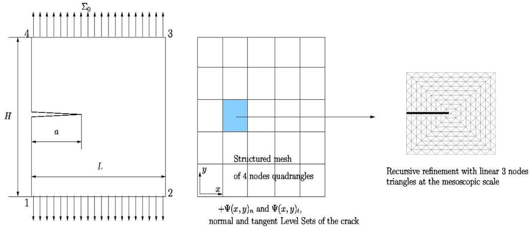
Figure 3: A standard 2D sample submitted to uni-axial loading.
