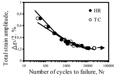
Figure 2: Total strain amplitude ( $\Delta\epsilon_t/2$ ) vs. Number of cycles to failure ( $N_f$ ) curves.
