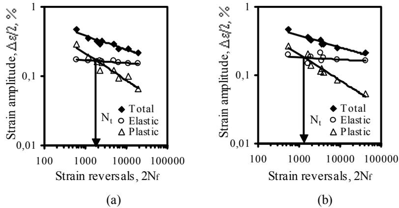
Figure 3: Elastic and plastic components of the total strain vs. strain reversals for (a) the hot rolled and (b) the tempered bars.
