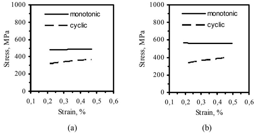
Figure 4: Monotonic and cyclic stress-strain curves for (a) the hot rolled and (b) the tempered bars.
