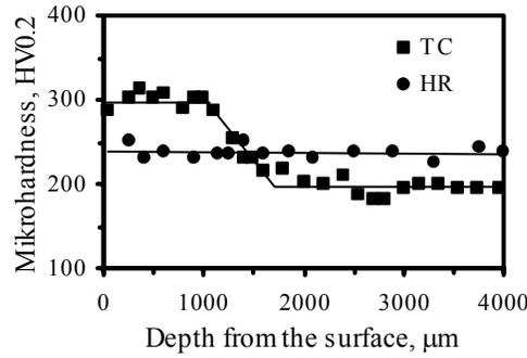
Figure 1: Hardness distribution throughout the cross section of the samples.
