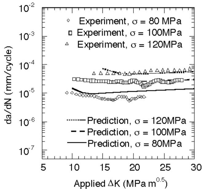
Figure 5. Comparison of model predictions and experimental data for a GLARE laminate at three stress levels.
