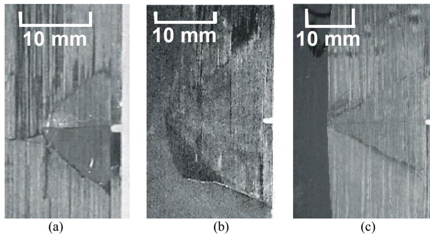
Figure 2. Delamination geometry in TiGr hybrid laminate revealed by use of a penetrant at fatigue crack lengths of: (a)  $a=8.7$  mm, (b)  $a=19$  mm and (c)  $a=23$  mm. The damage initiated from the small notches to the right of the figure.
