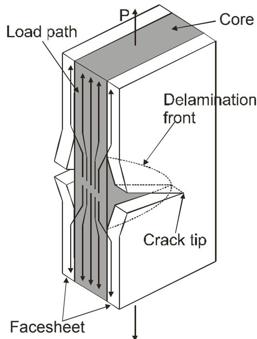
Figure 3. Schematic showing cracks in a metal foil accompanied by delamination from the polymer-matrix composite plies.
