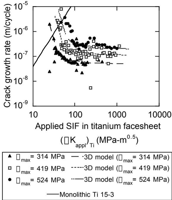
Figure 4. Comparison of model predictions and experimental data for (Ti/0/90/0<sub>2</sub>)<sub>s</sub> loaded at three stress levels, R= 0.1.
