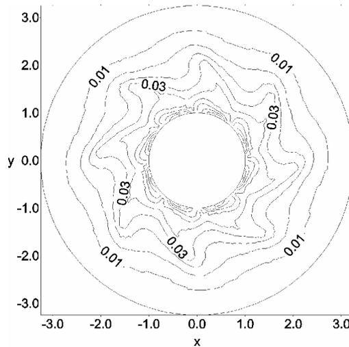
Figure 2: Isolines of maximum tangential stress.
