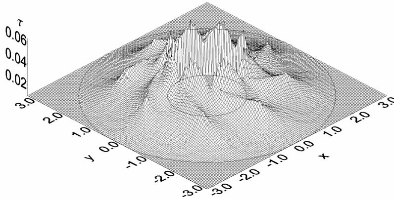
Figure 1: Surface of maximum tangential stress  $\tau(x,y)$ .
