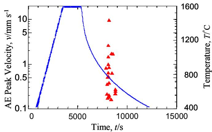
Fig. 5 Typical AE behavior during sintering of alumina detected by laser AE technique.
