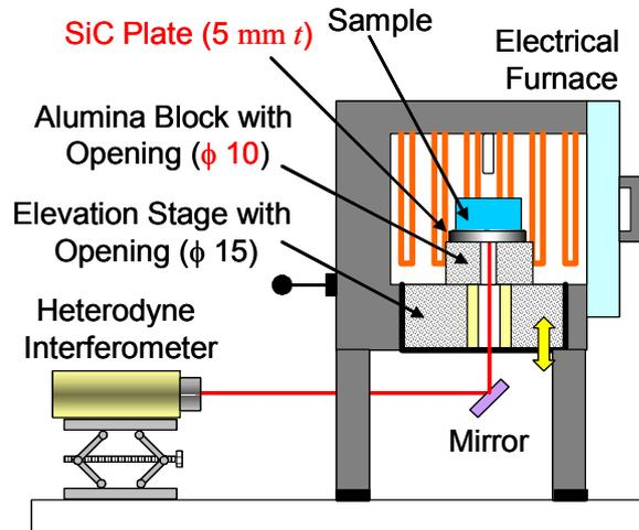
Fig. 2 Schematic figure of in-process monitoring system using laser interferometer for sintering of ceramics.
