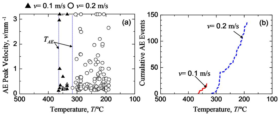
Fig. 4 Relationship between the (a) amplitude or (b) cumulative AE event and generation temperature of AE for different traverse speed of spraying gun.
