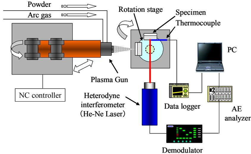
Fig. 1 Schematic figure of in-process monitoring system using laser interferometer for plasma spraying.
