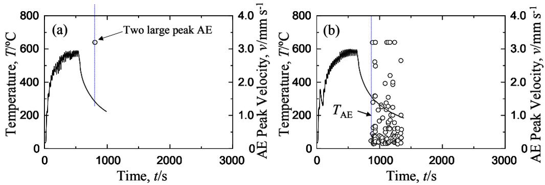
Fig. 3 Relationship between temperature history and AE behavior for different thickness of bond coat, (a)  $d_{BC} = 0$  mm and (b)  $d_{BC} = 70$   $\mu\text{m}$
