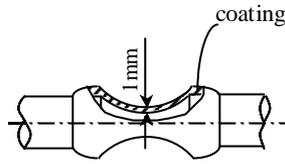
Fig.2 Schematic illustration of sprayed coating
