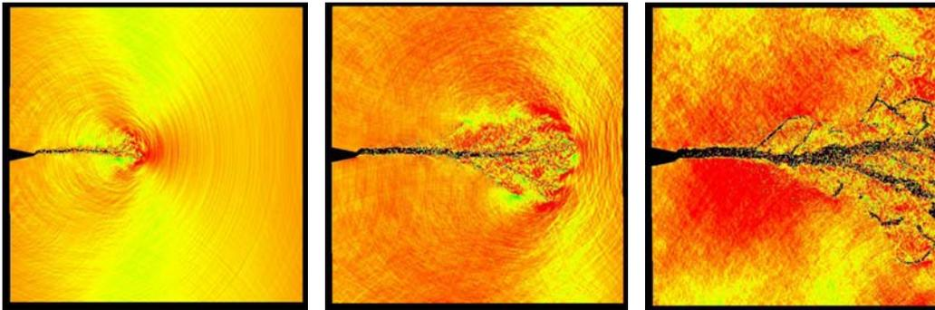
Figure 2. Snapshots (increasing times to the right) of the fracture process of a square pre-notched PMMA plate subjected to an initial uniform strain rate in the vertical direction.
