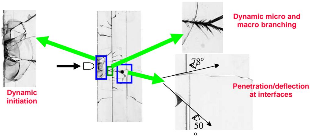
Figure 3. Phenomenon of catastrophic fragmentation: (1) dynamic crack propagation, curving and kinking, (2) triggering of branching instability, and (3) interaction of opening and shear dynamic cracks with interfaces (deflection/penetration).
