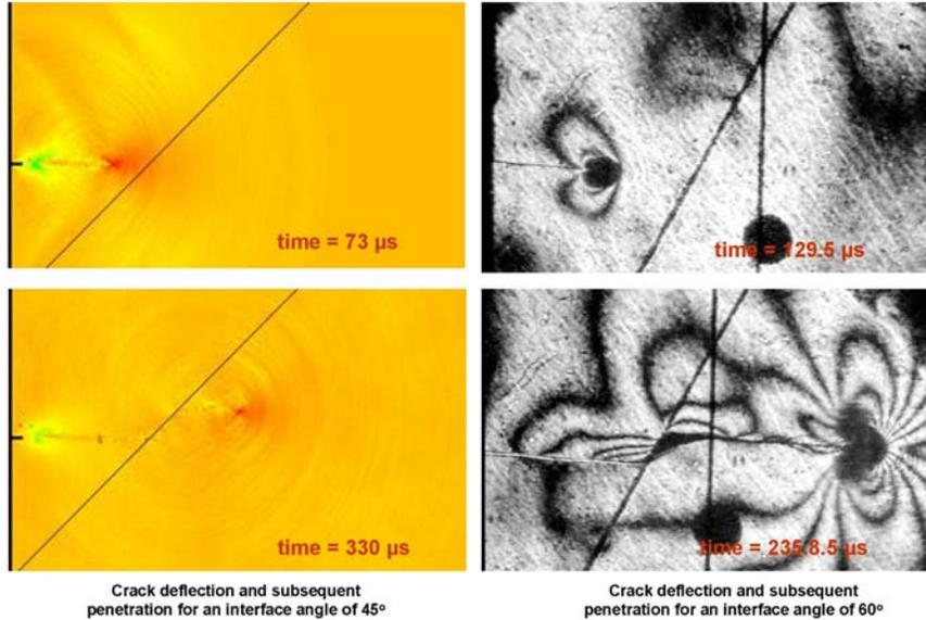
Figure 5. Qualitative comparison of deflection behavior in simulation (left) and experiment (right).
