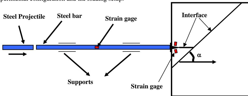
Figure 4: Modified Hopkinson bar loading setup.
