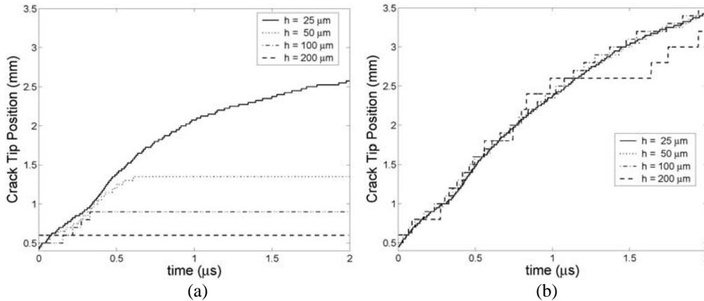
Figure 6. Double-cantilever beam test: solutions for under-resolved meshes with actual (a) and renormalized (b) cohesive parameters.
