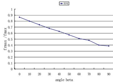
Figure. 4 Variation of  $f_{r\theta max}/f_{\theta max}$  with  $\beta$  under tensile-shear mixed loading
