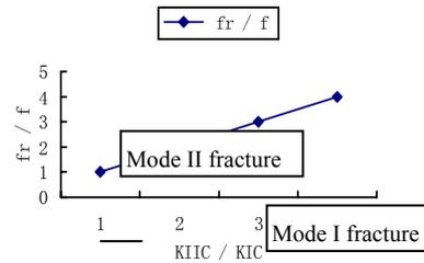
Figure.5 Fracture locus for occurrence of mode I or mode II fracture
