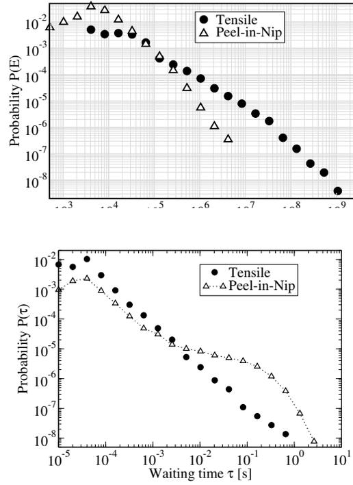
Figure 3: Top panel: the energy distribution  $P(E)$  for two experimental setups. Both exhibit *power-law* statistics, but with different exponents, and that the mode I has a much smaller exponent (close to 1.2). Lower panel: The distribution of time intervals  $\tau$  for the mode I and in-plane experiments. Both obey an Omori's law -like scaling, and the mode I one scales close to  $P(\tau) \sim \tau^{-1}$ . For the latter one there is a distinct time-scale (see text).
