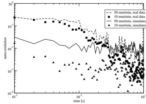
Figure 4: The autocorrelation function of released energy from the in-plane experiment, for two strain rates (10 and 50 mm/min). The data is compared to two artificial timeseries with the same interval and energy statistics.
