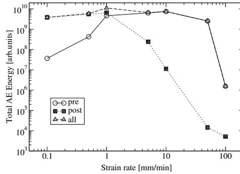
Figure 1: The fractions of AE energy, prior and after to the  $\sigma_c$  of the stress-strain curve, as a function of the strain rate in mode I experiments.
