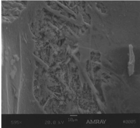
(a) Needle-like Ettringite Crystals
