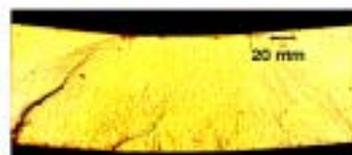
Picture 1 Multiple cracks in DFRCC
