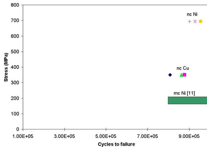
Figure 6: Fatigue test results for nc Cu and nc Ni. Also shown are the values for mc Ni from literature for comparison [11].
