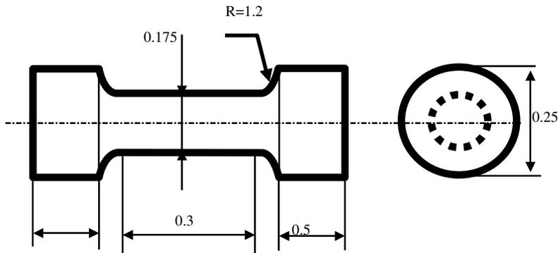
Figure 2: Specimen geometry and dimensions for fatigue test specimens.
