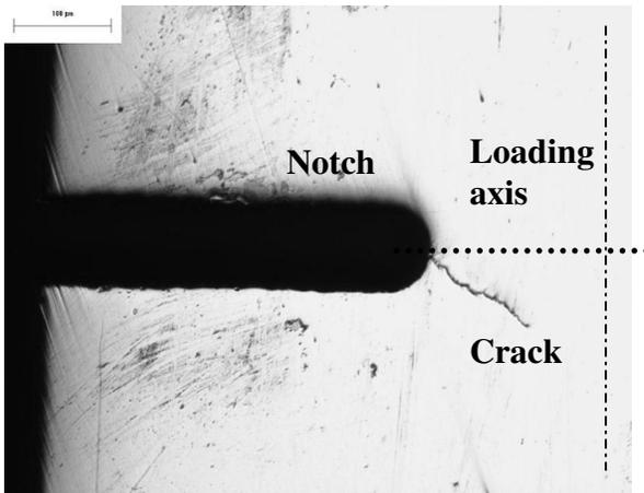
Figure 4: Optical micrograph of fatigue precrack at an angle to the loading axis.
