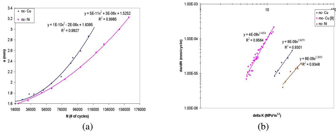
Figure 3: (a) Plot of crack length vs. number of cycles for nc Cu and nc Ni. (b)  $da/dN - \Delta K$  curves for copper and nickel.
