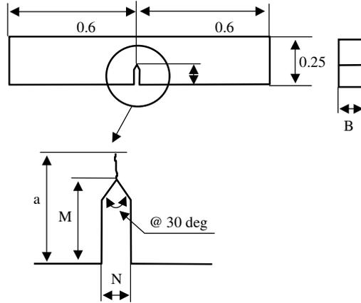
Figure 1: Specimen geometry and dimensions of the SENB fracture toughness specimens.
