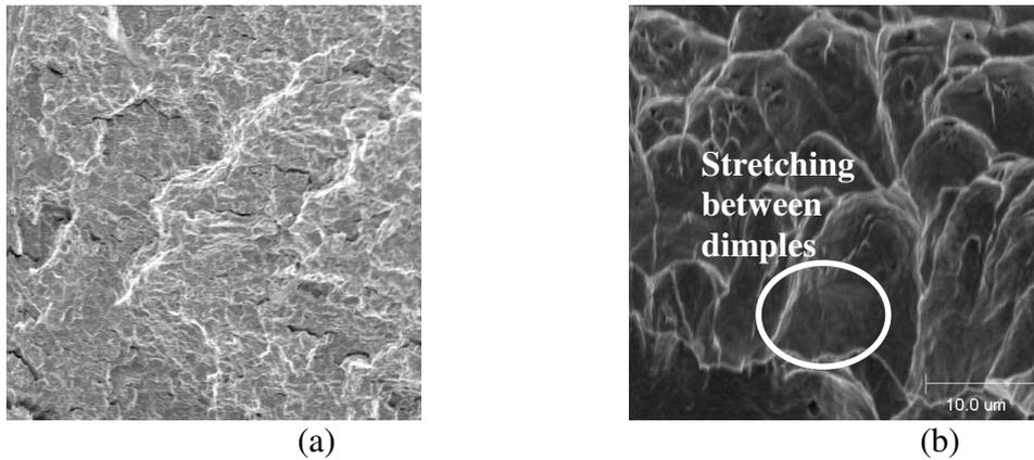
Figure 5: SEM micrographs of fracture surface for copper at (a) lower and (b) higher magnifications
