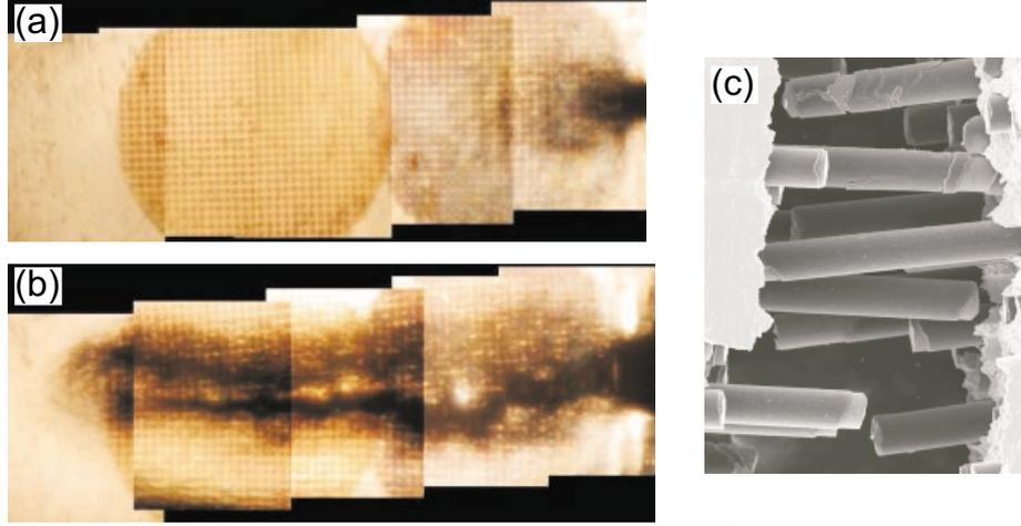
Figure 2.(a) and (b) Optical images of the fracture process zone. (c) SEM image of the crack showing fiber bridging and pull-out.
