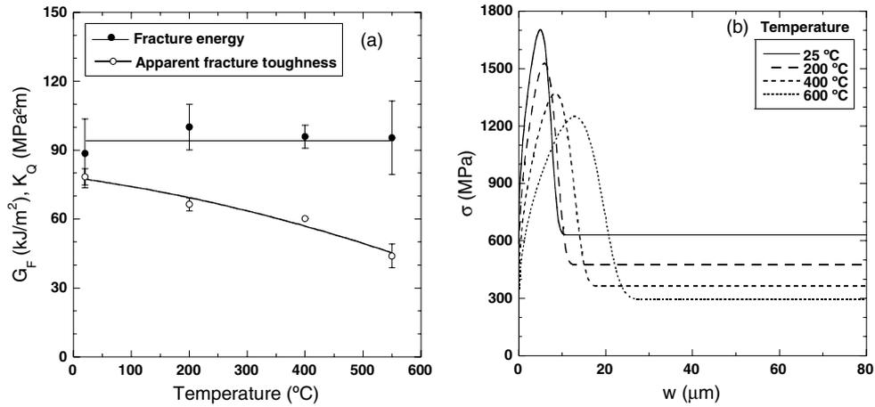
Figure 3 (a). Fracture energy and apparent fracture toughness of the TiSiC composite. (b) Cohesive curves as a function of temperature.
