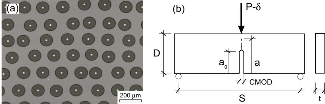
Figure 1. (a) SEM image of the cross section of the composite panel. (b) Geometry of the TPB specimens used in the fracture tests.
