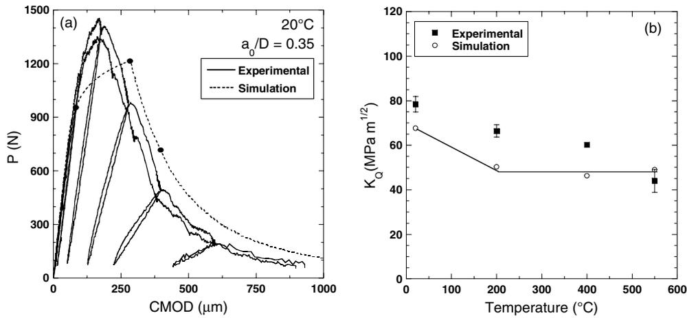
Figure 4 (a). Numerical and experimental results of the P-CMOD curves at room temperature for a beam with  $a_0/D=0.35$ . (b) Numerical and experimental apparent fracture toughness,  $K_Q$ , as a function of temperature.
