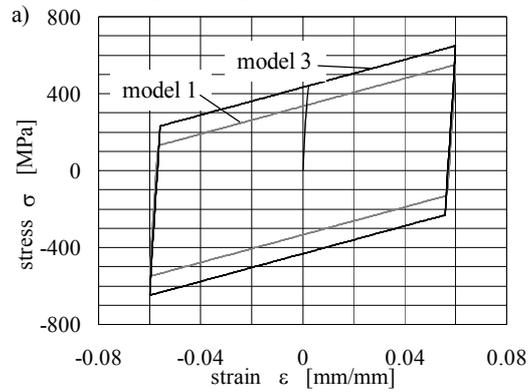
Figure 2: Cyclic stress strain curve of model 1 and 3
