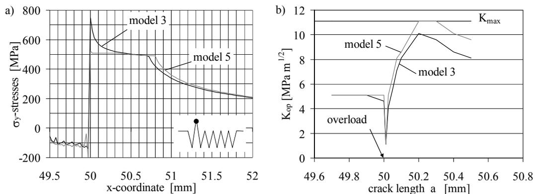
Figure 5: Comparison of the effects of bilinear and ideally plastic stress-strain behaviour
