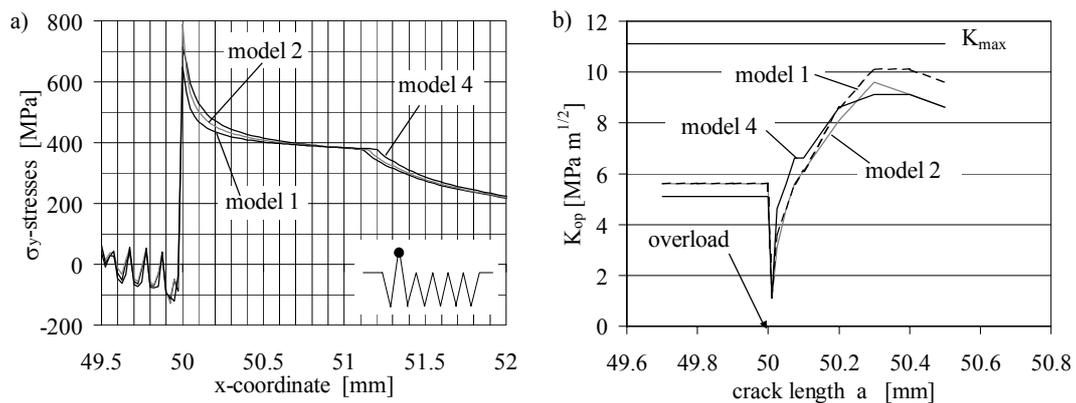
Figure 7: Influence of the investigated kinematic hardening parameters on the  $\sigma_y$ -stress distribution at  $K_{ol}$  at  $a = 50.0$  mm
