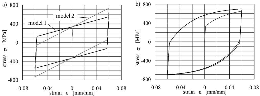
Figure 6: Cyclic stress-strain curve a) of model 1 and 2 and b) of model 4
