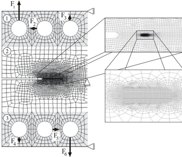
Figure 1: FE-model of the used CTS-specimen with a magnification of the interesting region
