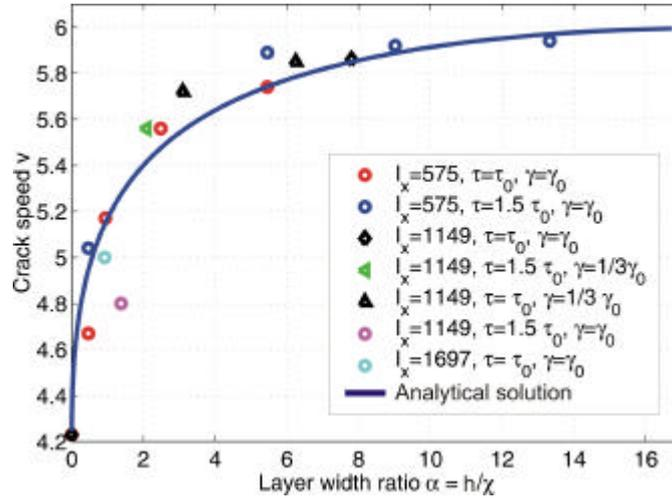
Fig. 3: Comparison of MD simulation results with the analytical solution to the mode III Broberg problem.
