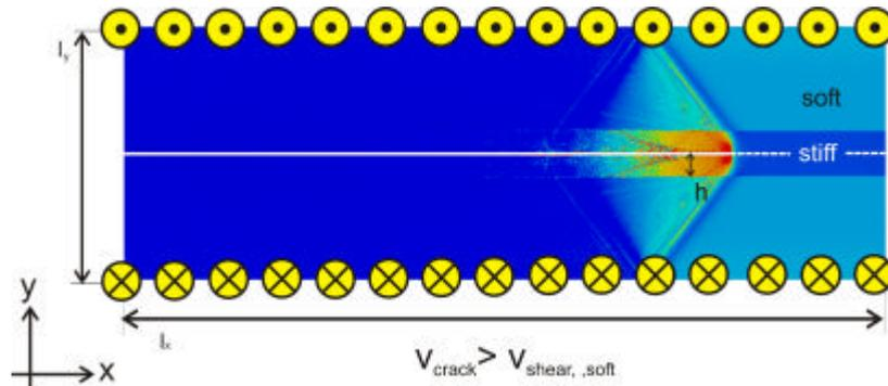
Fig. 1: Geometry of supersonic mode III crack propagation in a stiff layer surrounded by a soft matrix. The plot shows the potential energy field. The Mach cone due to supersonic crack motion is clearly visible in the soft matrix.
