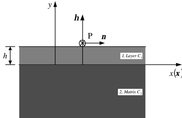
Fig. 2: Model of a concentrated force  $P$  moving with a constant velocity  $v$  acting on  $y = h$
