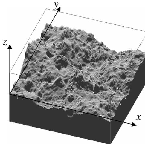
Figure 2: Topography of a mortar fracture surface. The side length of this map is 130 mm.
