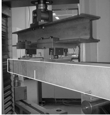
Figure 1: Mortar beam. The outline and the initial notch have been underlined for clarity.
