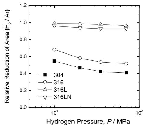
Figure 2. Effect of hydrogen pressure on relative reduction of area of type 304, 316, 316L and 316LN stainless steels at room temperature.
