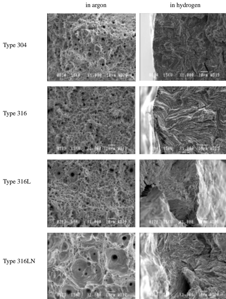
Figure 3 Fracture surfaces of type 304, 316, 316L and 316LN stainless steels in 70 MPa hydrogen and in argon at room temperature.
