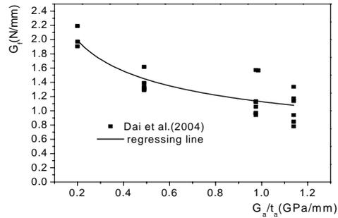
Figure 3 effects of adhesive layer on  $G_f$
