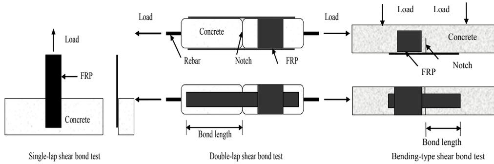
Figure 1 conventional shear bond test for FRP laminate-concrete interfaces
