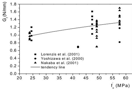
Figure 2 effects of concrete strength on  $G_f$
