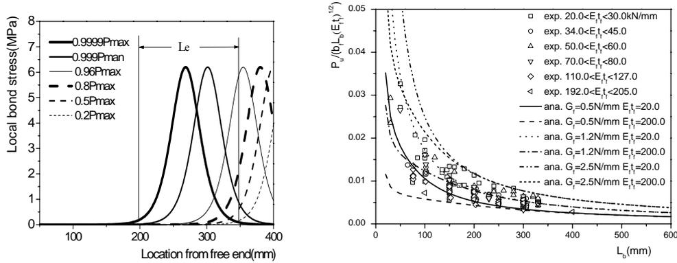
Figure 6 definition of the effective bond length  $L_e$  Figure 7 average bond strength  $\sim L_b$  relationship
