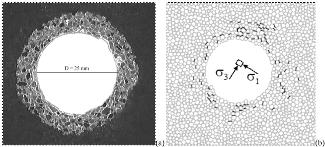
Figure 3: Crack pattern from a 2-mm specimen type B after testing to an external pressure of 38 MPa. Shown is the damage zone being lighter in color than surrounding intact material and the cracks tinted in white (a). Section from the PFC<sup>2D</sup> hollow-cylinder model of 4451 arbitrarily sized particles and 9582 contacts. Shown is the crack pattern developed at an external pressure of 38 MPa as short black lines (b).
