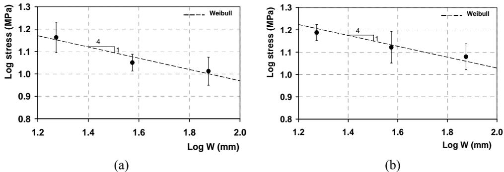
Figure 2. Bi-logarithmic plot for stress versus wall thickness, specimens A, B, and C. Shown are mean values and standard deviation for the 2 mm mixture (a), and the 4 mm mixture (b).
