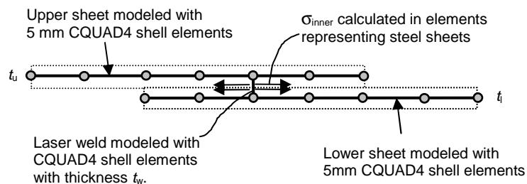
Figure 2: FE representation of laser weld joints and location for evaluation of structural stress.
