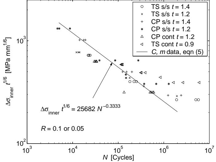
Figure 4: Stress-life results for test results in Fig. 1:  $\Delta\sigma t^{(m-2)/2m}$  data, and derived fatigue life curve for input to stress-based, fatigue life prediction software FE-Fatigue [2].
