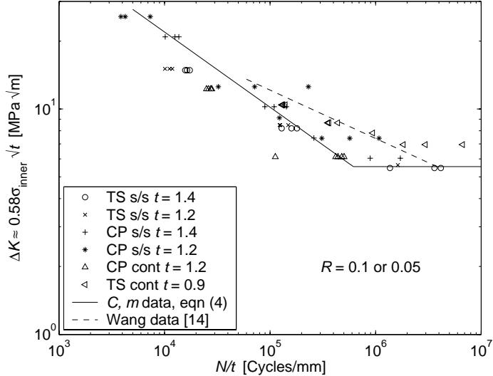
Figure 3: SIF-life results for test results in Fig. 1:  $\Delta K \approx 0.58\Delta\sigma_{\text{inner}}\sqrt{t}$  data, derived fatigue life curve using 95% crack growth data by Hobbacher [13], and fatigue data by Wang [14].
