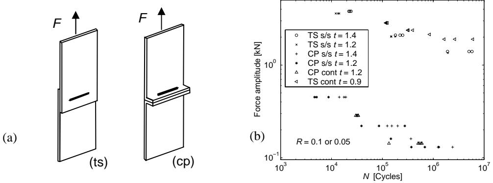
Figure 1: Fatigue data for different laser welded steel specimens: (a) Schematics of shear and peel loaded specimens; (b) Fatigue data for the different specimens in (a).
