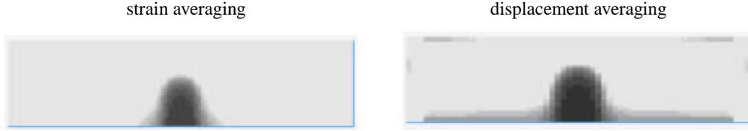
Figure 1: Distribution of damage in the three-point bending test obtained by nonlocal damage models with strain averaging and with displacement averaging (using the standard weight function)
