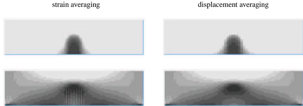
Figure 2: Distribution of damage (top) and stress  $\sigma_{xx}$  (bottom) in the three-point bending test obtained by nonlocal models with strain averaging and with displacement averaging (using the modified weight function)
