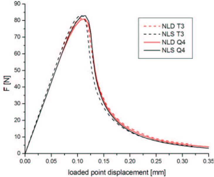
Figure 3: Load-displacement curves for different models and meshes (NLD = nonlocal displacement, NLS = nonlocal strain, Q4 = quadrilateral mesh, T3 = triangular mesh)
