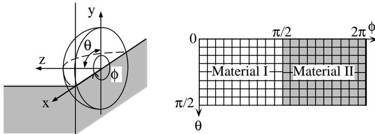
Fig.8 Model for eigen analysis (3D-line analysis)
