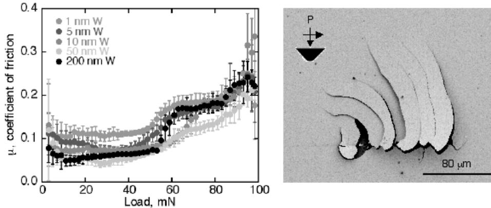
Figure 2. Nanoscratch tests using a conical indenter show that (a) frictional response varied with film thickness. (b) At loads near 50 mN, these tests triggered channel cracking and delamination as shown for the 200 nm thick ALD tungsten film.
