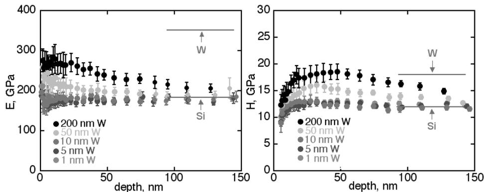
Figure 1. (a) Elastic modulus and (b) hardness increased with film thickness. The values were higher than those of the silicon substrate. Bulk tungsten and silicon substrate values are shown for comparison.
