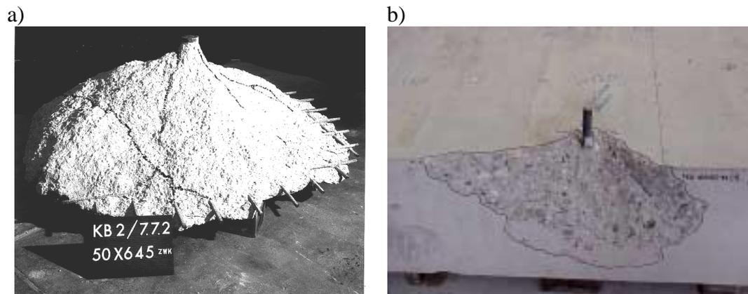
Figure 1: Typical concrete breakout cone obtained in the tests for: (a) tensile load and (b) shear load (Eligehausen et al. [1]).
