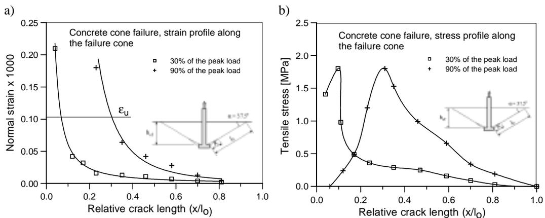
Figure 3: (a) The relative crack length at 30% and 90% of the ultimate load and (b) Distribution of stresses along the concrete cone surface at 30% and 90% of the ultimate load,  $h_{ef} = 520$  mm (Eligehausen and Sawade [8]).
