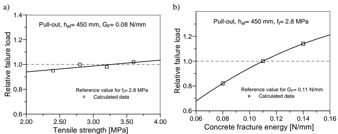
Figure 5: (a) Nominal pull-out strength as a function of concrete tensile strength (Ožbolt [3]); (b) Nominal pull-out strength as a function of concrete fracture energy (Ožbolt [3]).
