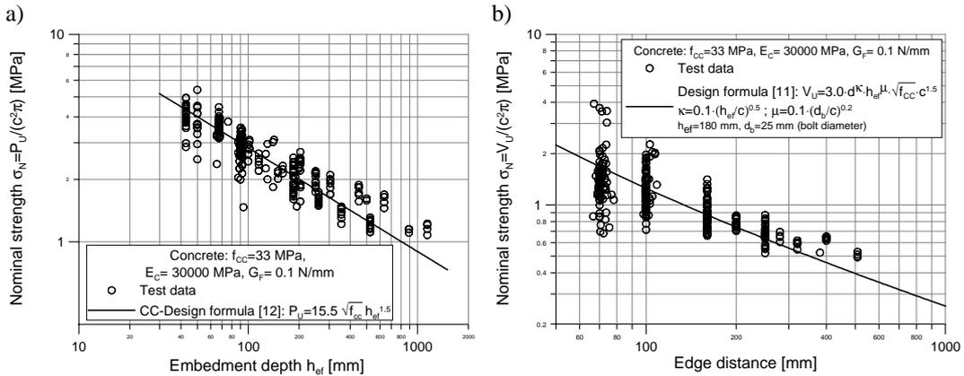
Figure 6: Concrete cone breakout - summary of experimental results and comparison with proposed design formula based on the LEFM: (a) nominal pull-out cone strength and (b) nominal shear cone strength.
