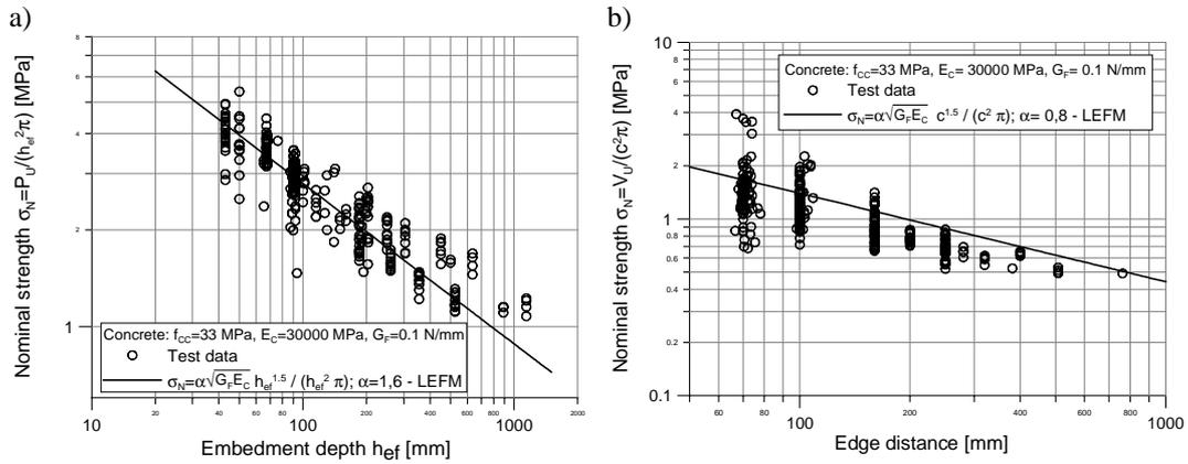
Figure 2: Concrete cone breakout - summary of experimental results and comparison with LEFM based formula for: (a) nominal pull-out concrete cone strength and (b) nominal shear cone strength.
