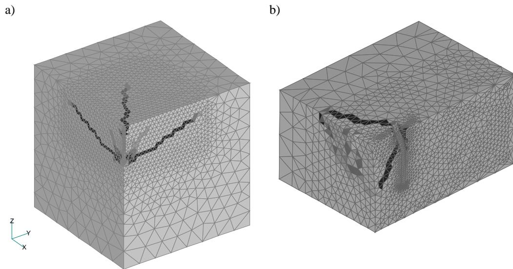
Figure 4: Typical failure modes obtained from the 3D finite element analysis: (a) tensile load and (b) shear load.
