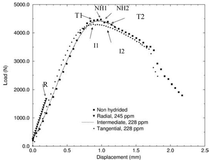
Figure 3: Load-displacement curves obtained from macroscopic tensile tests for non-hydrided and hydrided material (roughly 230ppm) with 3 different hydrides orientations.
