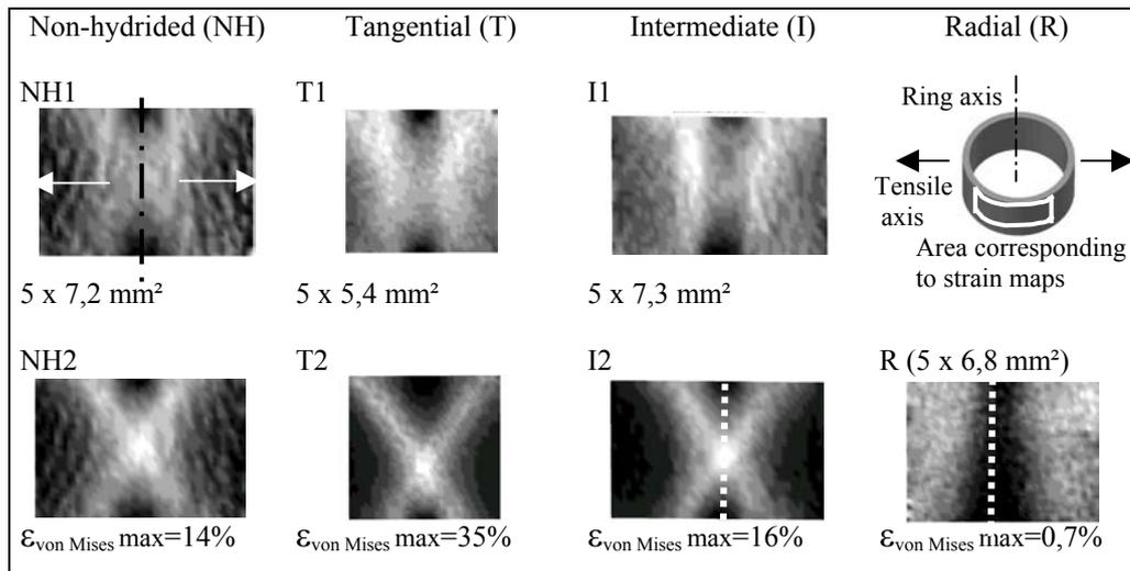
Figure 4: Strain maps of the different materials studied before and after the localization strain bands apparition (if any). The maximal deviatoric strain value is given by the highest gray level (white color). In the last two cases the dotted line represents the crack path.
