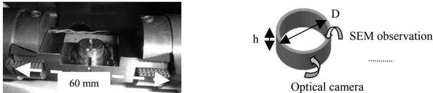
Figure 2: Ring testing system (left) and scheme of the ring with the observed surfaces (right)
