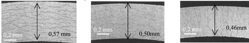
Figure 1: Metallographic cross sections of hydrided tubes (about 230ppm) with tangential (left), “intermediate” (middle) and radial hydrides (right).
