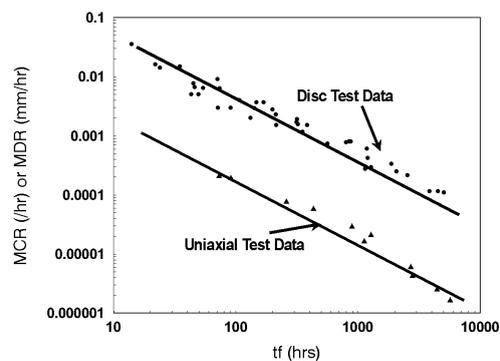
Figure 4: Data showing the Monkman-Grant relationships for uniaxial and disc SP tests on power station low alloy steels.
