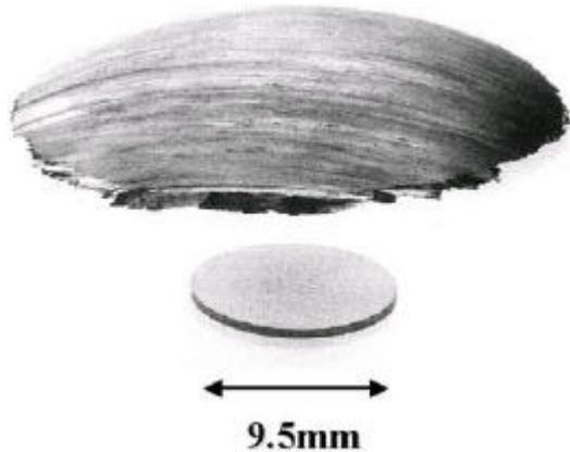
Figure 1: An example of a “scoop” cut with a hemispherical cutter next to an SP test specimen.
