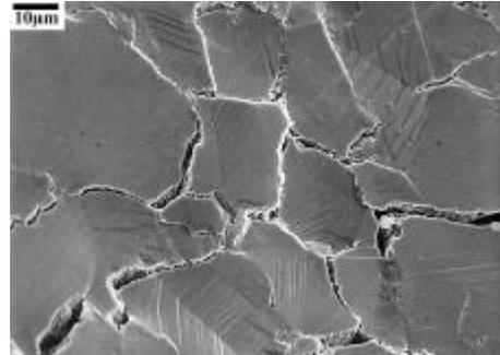
Figure 5b: Micrograph of the surface of an interrupted disc SP specimen showing grain boundary creep cavitation.
