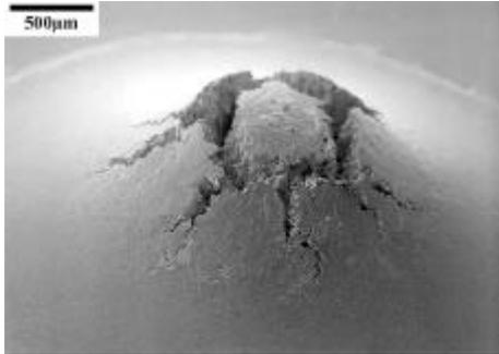
Figure 5a: Surface of bulged SP disc interrupted during testing.
