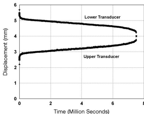
Figure 3: An example of the time/displacement data acquired from a creep SP test.
