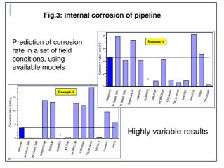
often observed (mesa corrosion), whose velocity can vary of more than one order of magnitude in different situation. Models are available and under development to calculate the corrosion rate as a function of the main parameter which can be measured and/or controlled during operations. In Fig.3 an example of the results from different models are shown. Two examples, referring each to a different field conditions, are shown.
