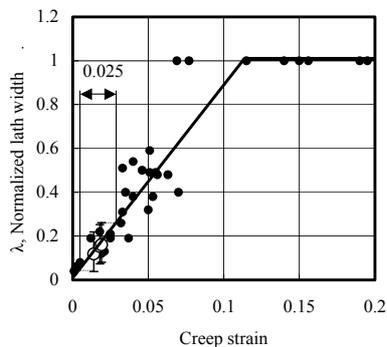
Figure 7. Comparison of the normalized lath width of ex-serviced products ( ) and the other martensitic advanced creep resistant steels ( ) with reference line.
