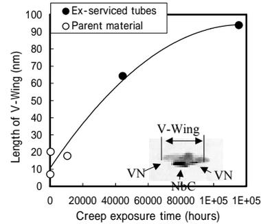
Figure 6. Monitoring of the length of V-Wing type
