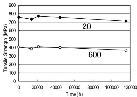
Figure 2. Stable tensile strength with exposure times for the tubes
