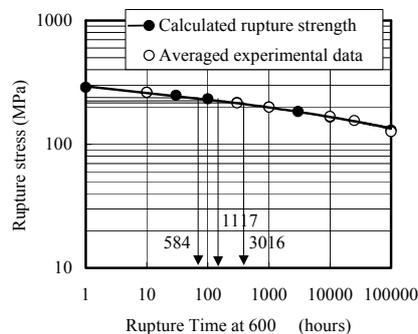
Figure 8. Agreement of the estimated creep rupture strength by Equation (1) with the experimental data
