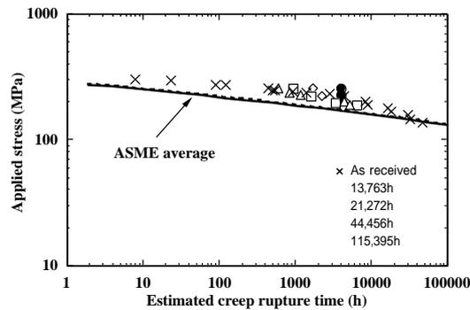
Figure 1. Creep resistance evaluation by extension creep for the ex-serviced tubes compared with that of the parent material at 600.
