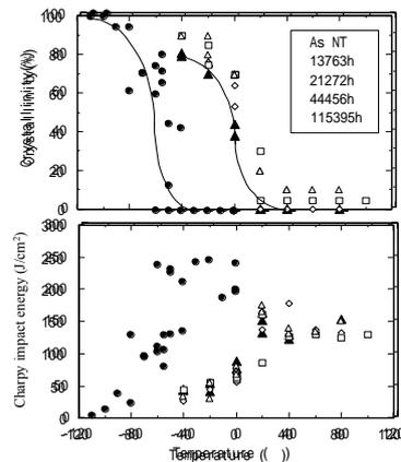
Figure 3. Charpy transition curves alteration with exposure times for the tubes.
