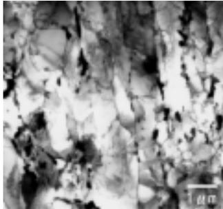
Figure 4-2. TEM image of the pipe after 64,363 hours exposure at steam temperature of 560 °C. A slight lath structure recovery is apparent.
