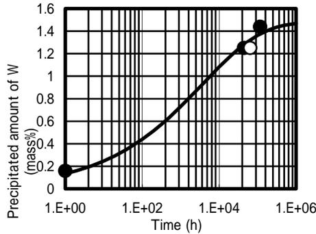
Figure 5. W precipitation during creep
