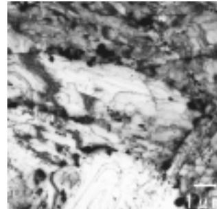
Figure 4-3. A sub-grain microstructure developed after 115,35 hours exposure at steam temperature of 569 °C.
