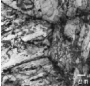
Figure 4-1. TEM image of thin foil for the tube after 44,456 hours in service at steam temperature of 569 °C.
