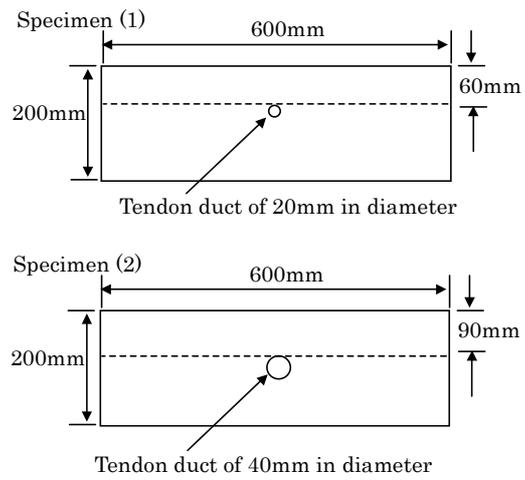
Figure 3: Concrete specimens.
