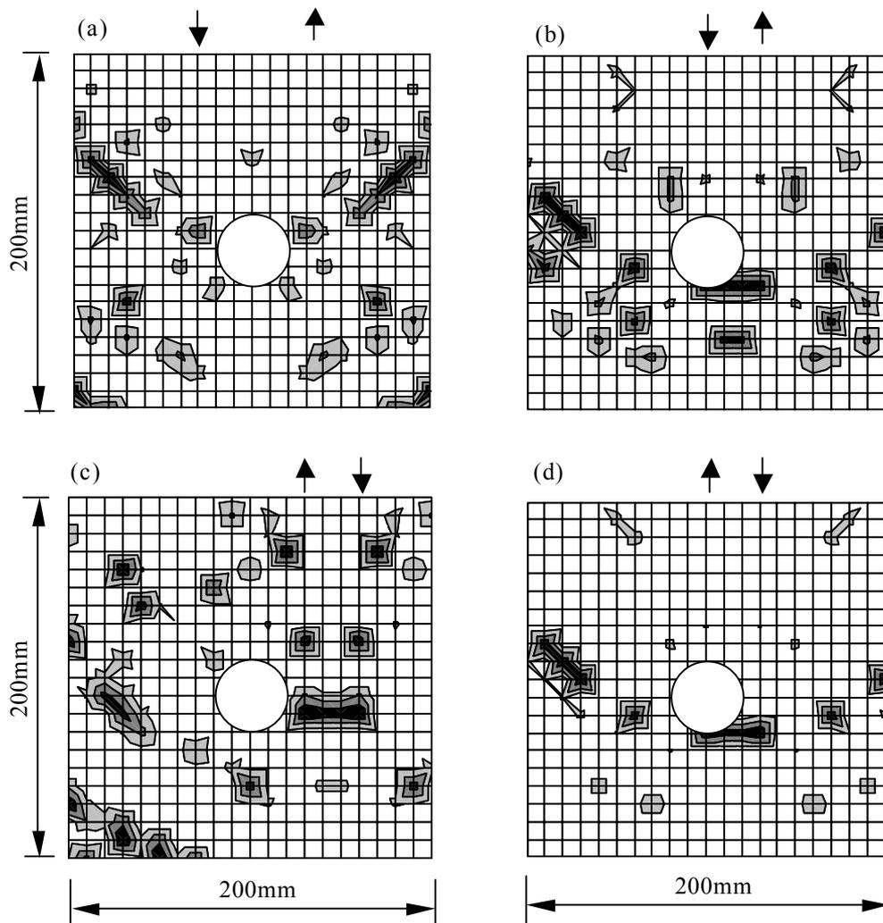
Figure 6: Results of SIBIE due to the specimen (2).
